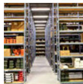
Very Narrow Aisle racking
